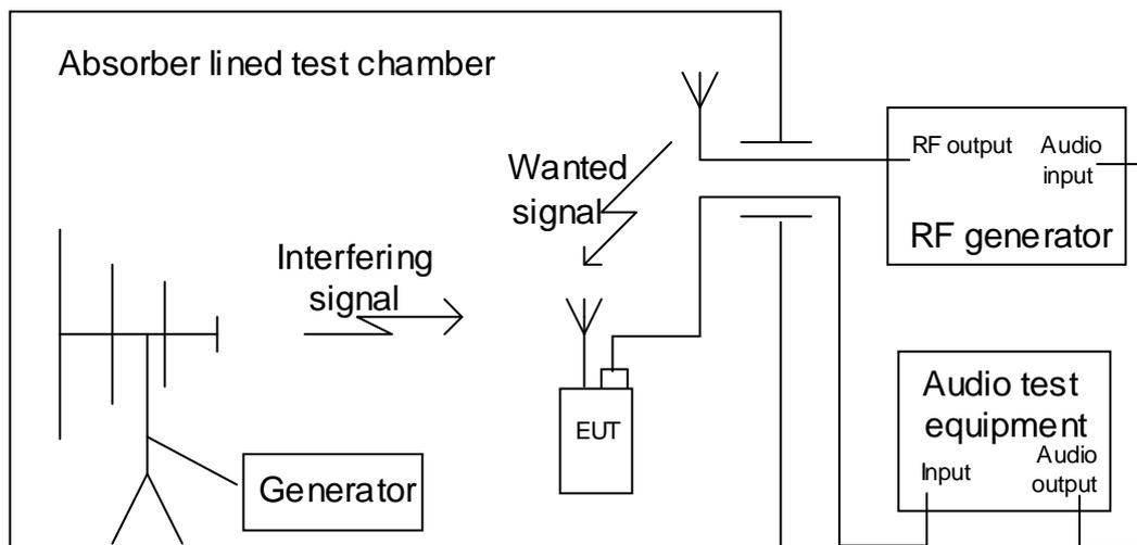
NOTE: The RF generator may be a companion transmitter sited inside the test chamber if necessary.
